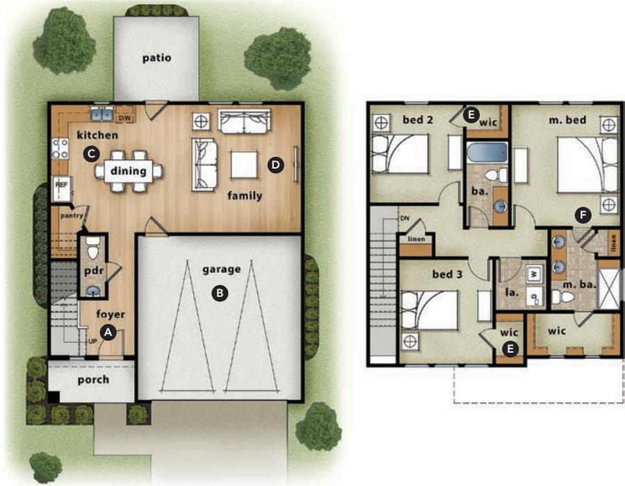
**T**his starter home is designed to achieve the perfect balance between livability and construction cost. All the floor framing runs in the same direction for the entire house, and it bears upon a wall running through the center of the home. The minimal breaks in the plan occur only on the front elevation to create breaks in the massing. This home is illustrated with both mid-century modern and Craftsman elevations to show the varied looks that can be achieved with the same floor plan.
