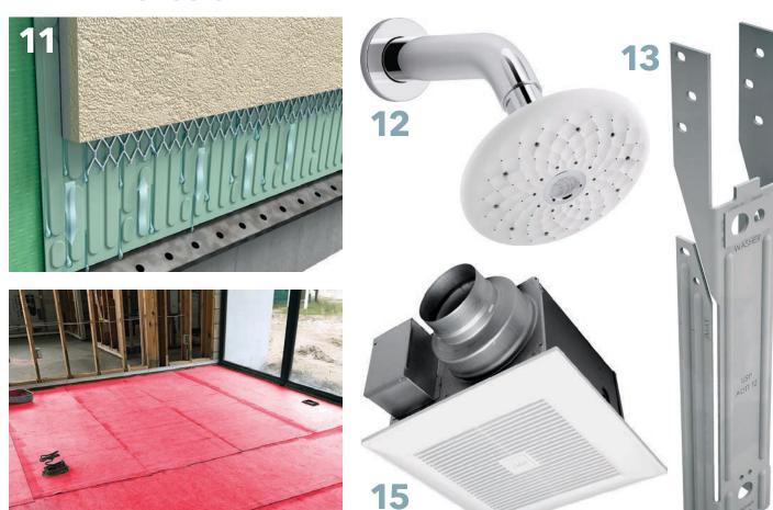
Water inevitably penetrates exterior cladding at some point. A practical way to handle that is to install **Kingspan** Greenguard DC14 drainage mat. Made of extruded polystyrene, DC14 doesn't absorb moisture. With drainage channels on both sides, it permits easy drainage for water and allows air movement between the siding and sheathing to help keep the wall dry. Also in The New American Home are the company's XPS insulation board and KoolDuct preinsulated ductwork. (Silver Sponsor)
