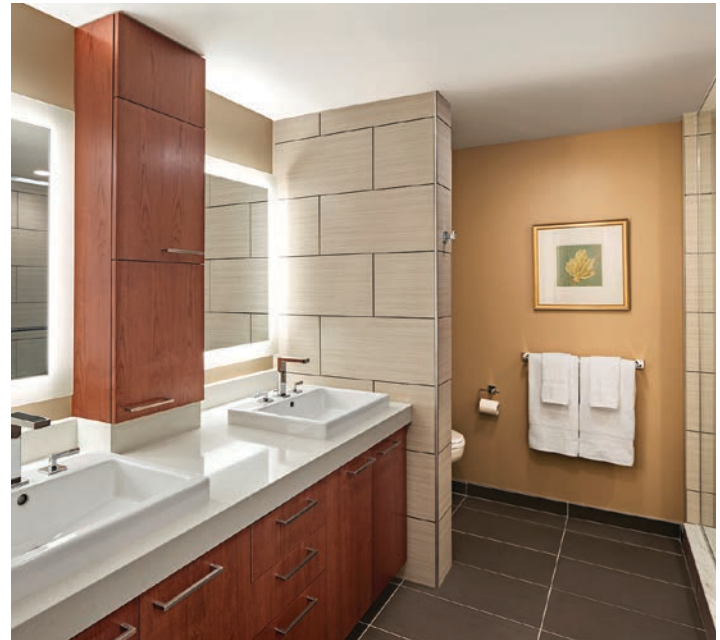
North Hill, a continuing care community in Needham, Mass., includes motion-sensor fixtures, contrasting surfaces, hospitality lighting, and handles that are easy to grasp.
